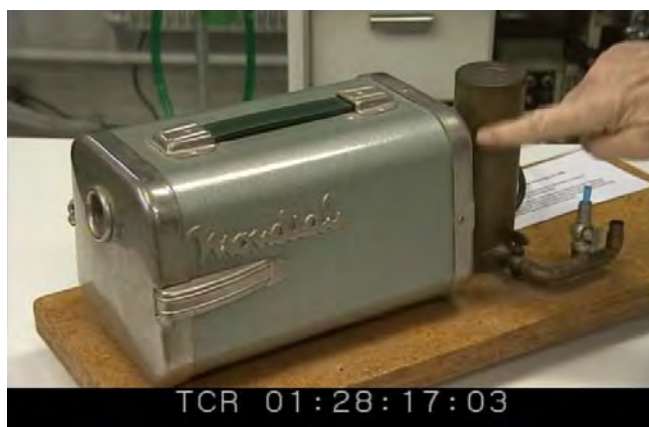
Fig. 1: Mondial vacuum cleaner transformed into a respirator for compressed air. Documented by an interview with the donor and constructor (Inv. 10226) 6 - Courtesy of the Institute of the History of Medicine, University of Berne and Inselspital-Stiftung Museum Collection.
