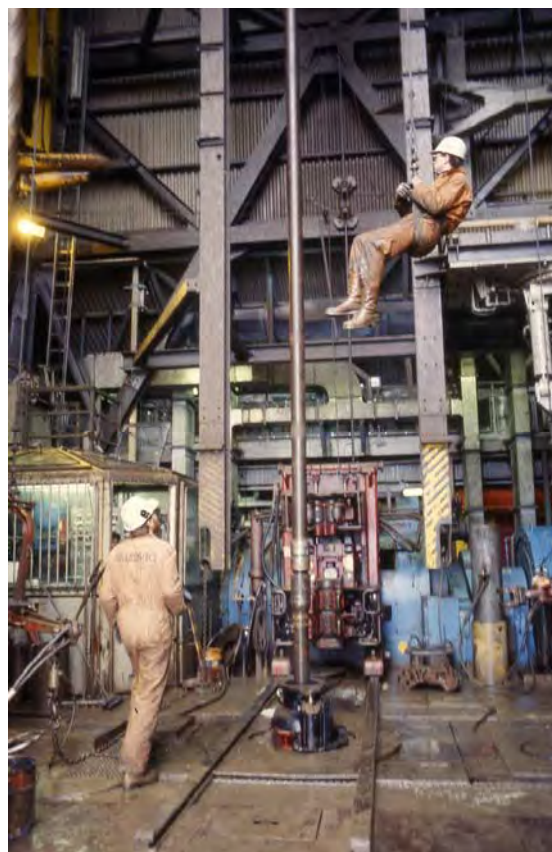
Fig. 4: A derrick man working above the drilling floor at Statfjord in the "old days". Photo: NPM.
