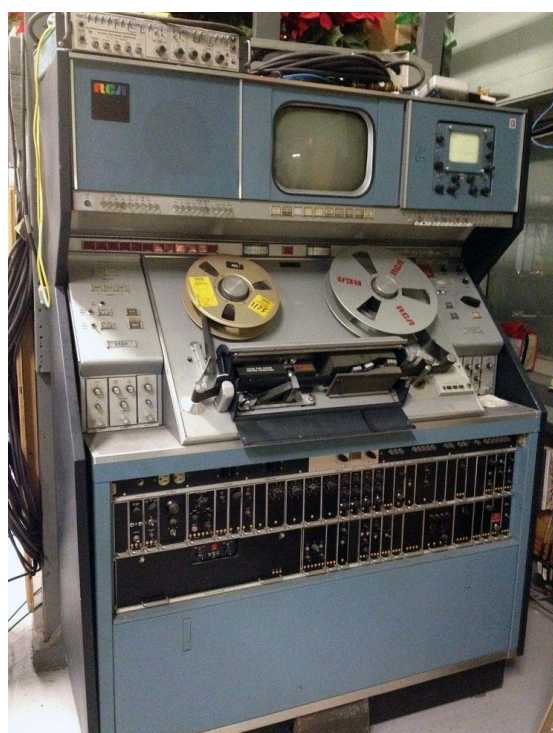
Fig. 2: An antique RCA TR-70C 2-inch Quadruplex Video Tape Recorder (VTR). The Vermont Public Television bought the 1,800 lb (approx. 820 kg) piece of equipment in 1976 and used it until 1991 (Photo credits: Vermont PBS).
