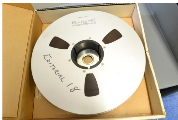
Fig. 1: Close-up of a larger 2" Quad open videotape reel.
